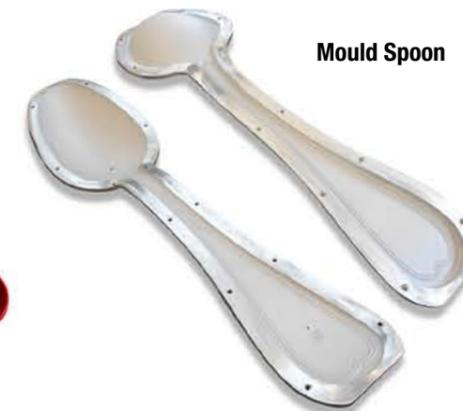
Then Persico prepared a CNC-milled aluminium mould for the production of the spoons. Finally, the actual 1.5-metre spoons were rotomoulded with Persico’s moulds using regenerated polyethylene plastic. The 63 huge spoons positioned on the front of the hotel in a target motif – red ones encircled by white – are a sight to behold.
